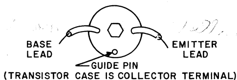
BOTTOM VIEW OF TRANSISTOR TYPE 2N442
